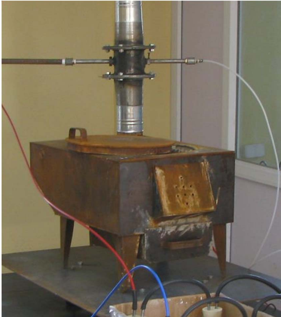
Typical traditional Mongolian cooking and heating stove with a sheet metal top.
